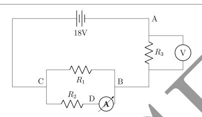
$R_{\rm CB} = 100\,\Omega$  and  $150\,\Omega$  parallel =  $60\,\Omega$
