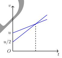
The area under each line gives the total displacement of the car. The cars will overtake each other when the area under both line are equal. The point of intersection of two lines is the instance when velocities are equal. Clearly, when velocities are equal, the total displacement of each car is different.
