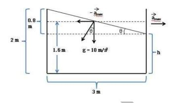
To find h, we equate the volumes in the two situations with changed geometry.
