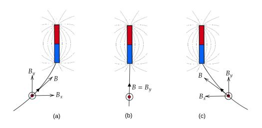
In this case,  $B_x$  is positive when the magnet is to the left of the magnetometer (a), zero when the center of the magnet aligns with the magnetometer (b), and negative (pointing left) when the magnet is to the right of the magnetometer (c). This is qualitatively depicted in the figure below.
