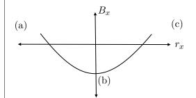
Orientation III will produce a graph that is the exact opposite of the previous one, with the signs of  $B_x$  reversed, as the dipole vector is now aligned in the -x direction. Let us consider another example with Orientation I, as shown in the figure below.
