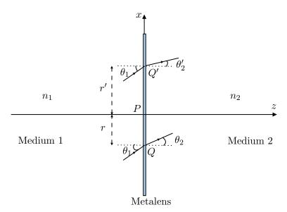
(a) [8 marks] Find f(r) in terms of  $\phi(r)$  and  $k_o$ , the wave number of the incoming wave in a vacuum. To determine f(r), assume two rays in x-z plane incident at an angle  $\theta_1$  at two infinitesimally close points, r and  $r + \Delta r$ , are refracted by the same angle  $\theta_2$ . You don't need to derive the exact functional form of  $\phi(r)$  for this part.
