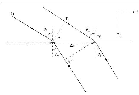
Consider two rays, which are close to each other, incident locally on metalens. The ray OA is incident at an angle  $\theta_1$  at r and exits in medium 2 at an angle  $\theta_2$ . Similarly the ray BB' exits in medium 2 at an angle of  $\theta_2$  from  $r + \Delta r$ . The rays being very close to each other have a plane wavefront. Let wavefront AB propagate to A'B' in time t. Let  $\psi_A, \psi_B, \psi_{A'}$  and  $\psi_{B'}$  be phases at points A, B, A' and B' respectively. Then
