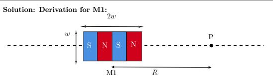
For M1, if we consider the pole strength to be m for each pole, the magnetic field at point P, which is at a distance r from the center of the magnet, can be expressed as:
