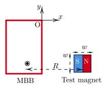
Figure 1: Schematic representation of the magnetic black box (MBB) and a test magnet.
