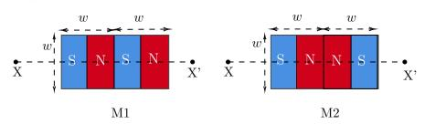
Figure 5: Magnetic sets M1 and M2. Here w = 10mm.
