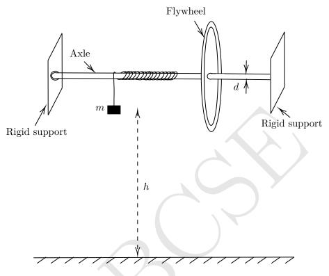
From the instant when the mass touches the floor (taken as t = 0), the flywheel continues to rotate, adding another N number of rotations before coming to rest in time t = T. The figure is not to scale.
