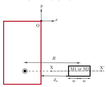
Figure 6: Setup for measuring the dipole moment.
