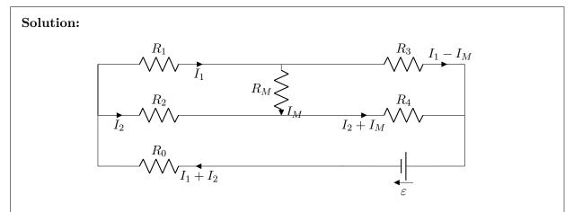
Resistances, currents and emf are shown in the diagram. Imagine also there is a resistance  $R_M$  between terminals 1 and 2. We can set later  $R_M = 0$  for an ideal ammeter and  $I_M = 0$  for an ideal voltmeter placed between two terminals. Applying Krichoff's law
