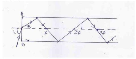
It is clear from the figure that the ray with incident angle i will get reflected from the mirror if X < 0 3X < d < 4X or 5X < d < 6X
