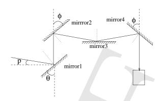
Let angle of incidences at the four mirrors be  $i_1$ ,  $i_2$ ,  $i_3$  and  $i_4$  respectively.
